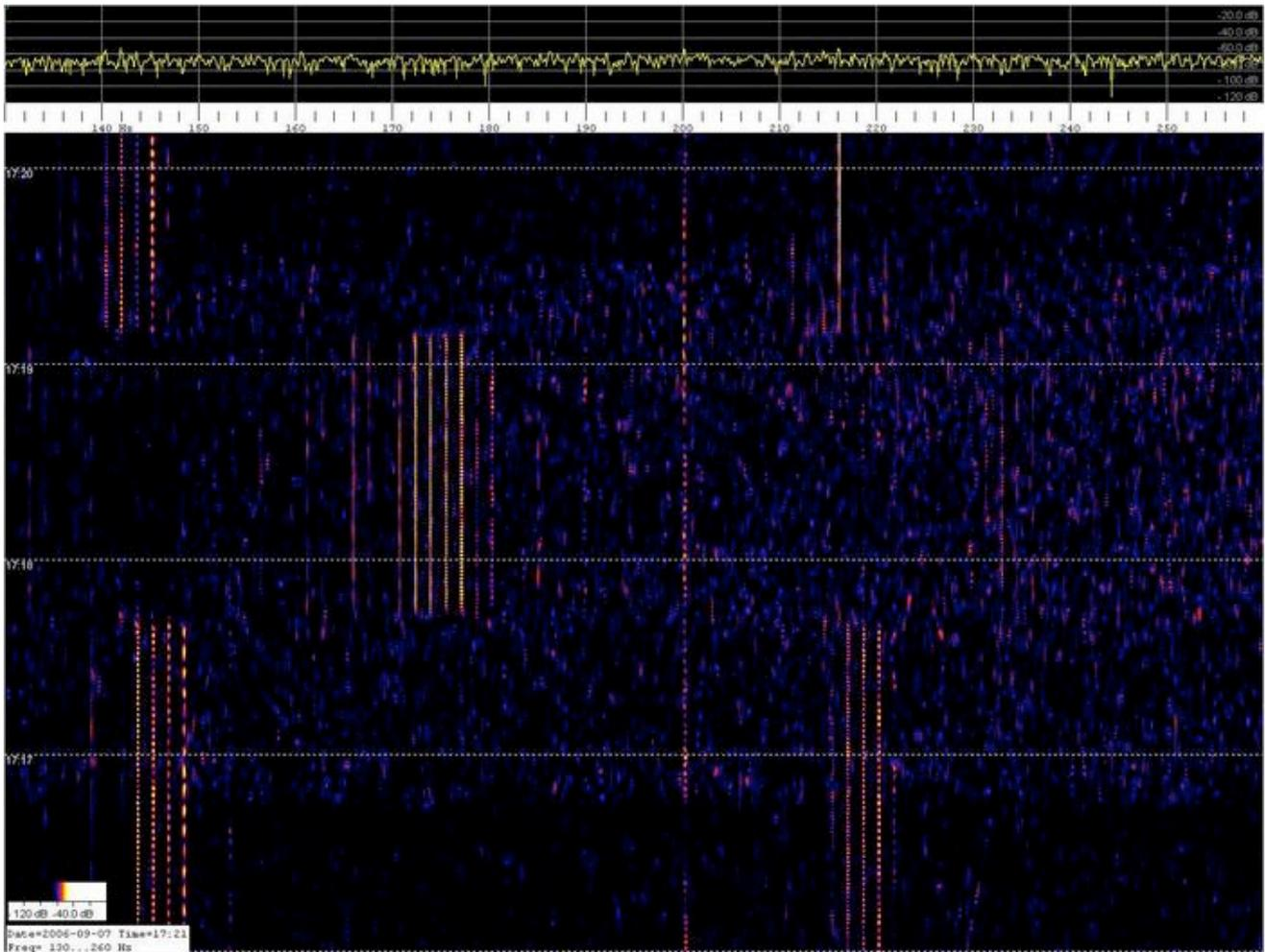
The image above shows a spectrum waterfall display<sup>16</sup> of the received audio signal. The difference between a candidate from the CDA (middle) and any other party (top and bottom) is clearly visible.
